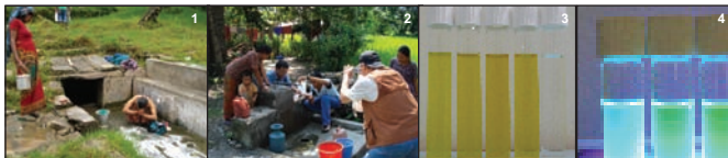
Fig. 2: Locals using shallow well (1), sampling from piped tap (2) using commercially available water test system. Out of five samples (tubes) four are positive for TC (3) and out of those four TC positive samples three (showing apple green color) are FC ( Esch. coli ) bacilli positive (4)
